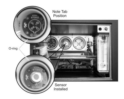
Figure 5-1: Sensor Block with Middle Sensor Installed
